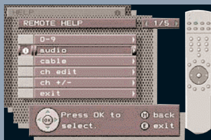
The remote control function menu with on-screen graphics describes the operation and functions of each button
