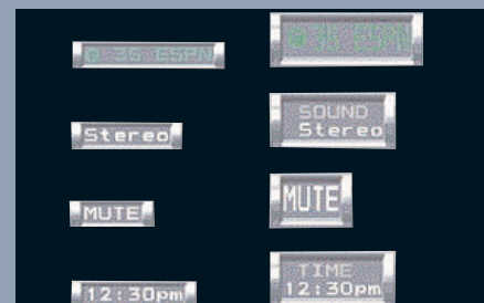
On-screen displays appearing each time the channel is changed can be configured for user preferences in size, screen position, and type of information
